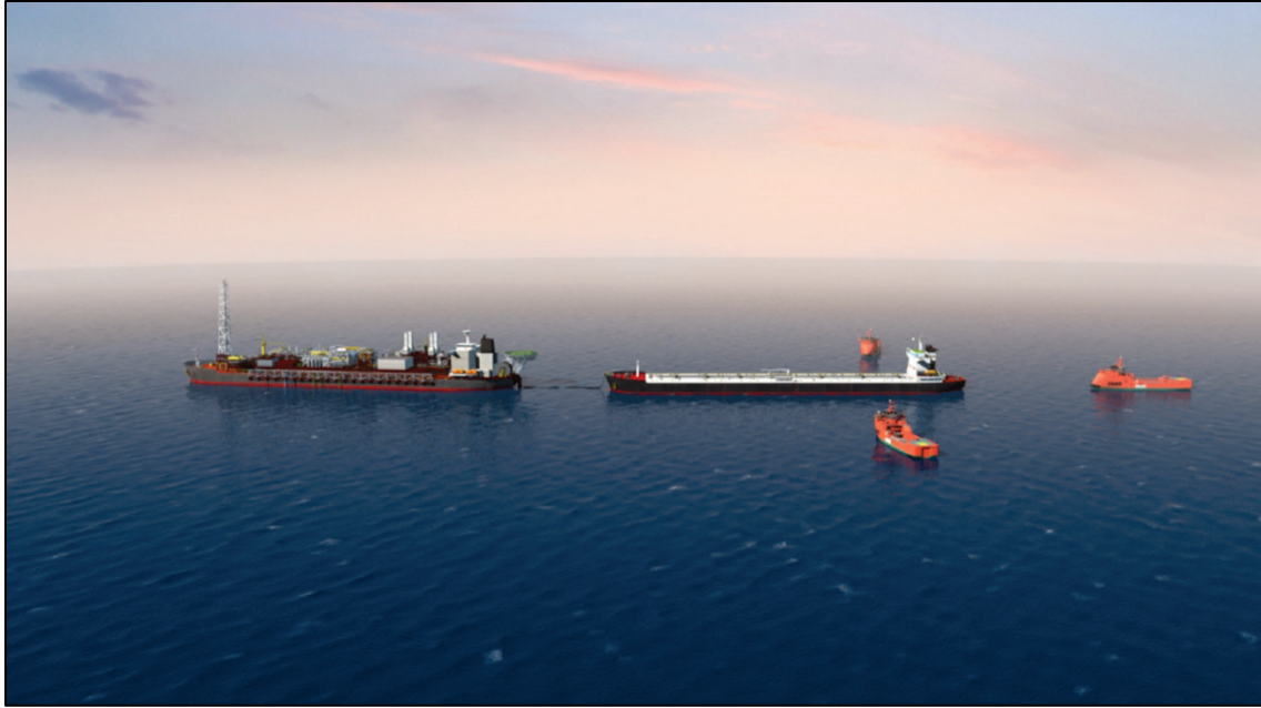
Figure 2.7-3: General Offloading Configuration
