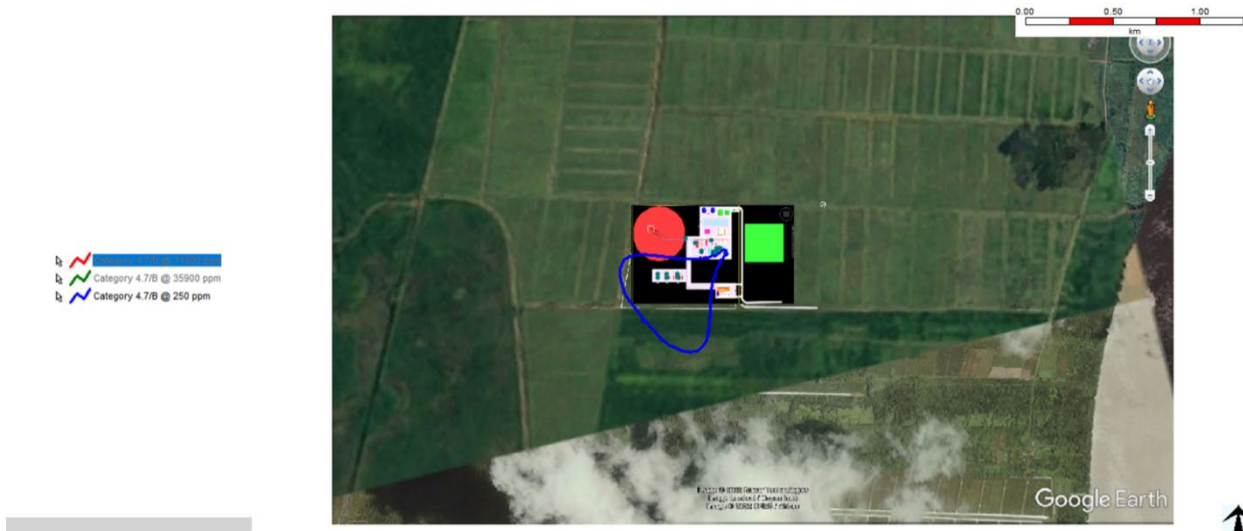
Figure 10.1-24: Flammable Cloud from Methanol Tank Release
