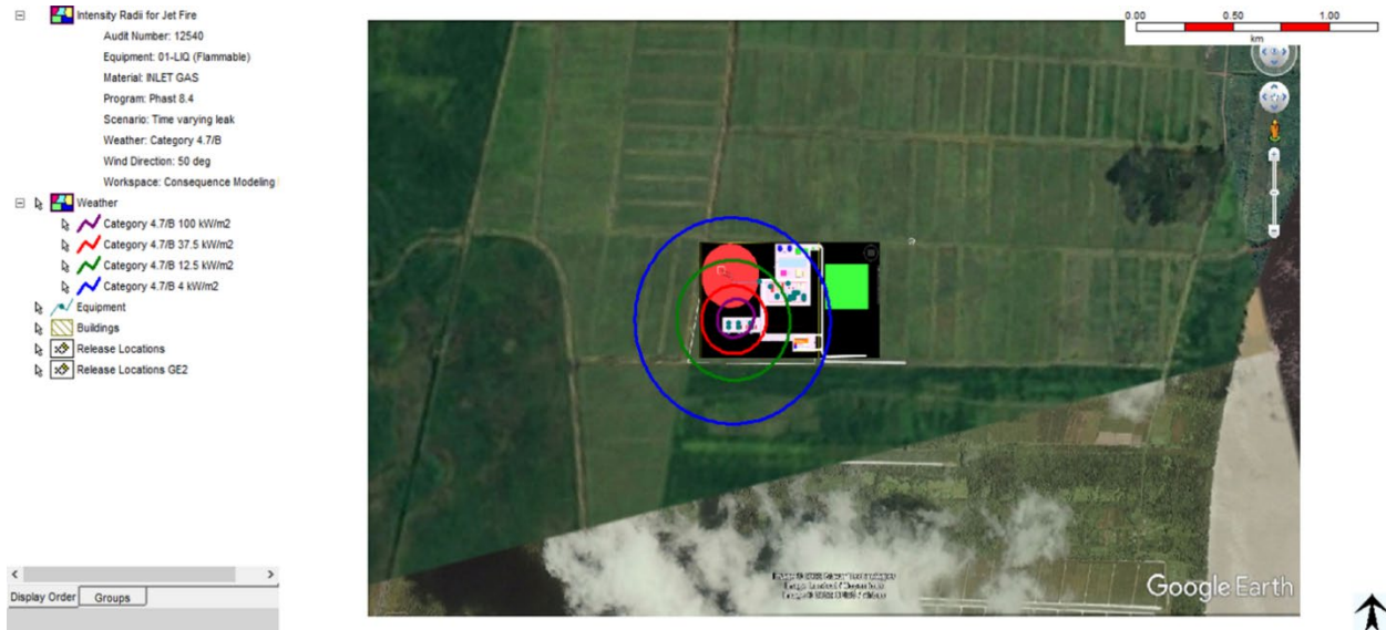
Figure 10.1-17: Jet Fire from Piping Upstream of Slug Catcher Natural Gas Release
