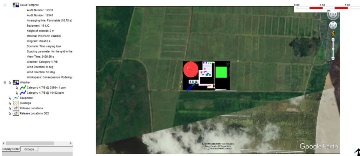
Figure 10.1-23: Flammable Cloud from Propane Storage Bullet Release
