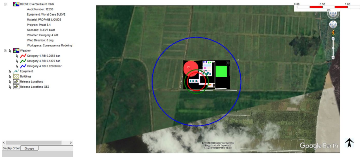
Figure 10.1-23: BLEVE from Propane Storage Bullet Release
