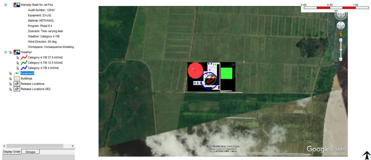
Figure 10.1-25: Jet Fire from Methanol Tank Release
