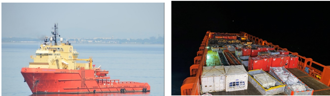
Figure 6-7: Marine Support Vessel and Typical Cargo Deck Configuration
