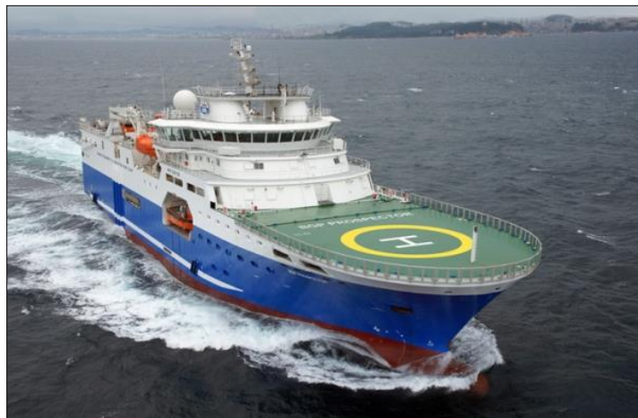
Figure 2: EXAMPLE OF A STREAMER VESSEL (BGP PROSPECTOR)
