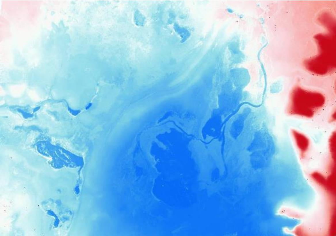
Figure 18: Digital Surface Model of the region represented in Figure 17. Red colour shows higher elevations while blue colour represents the lower elevations.
