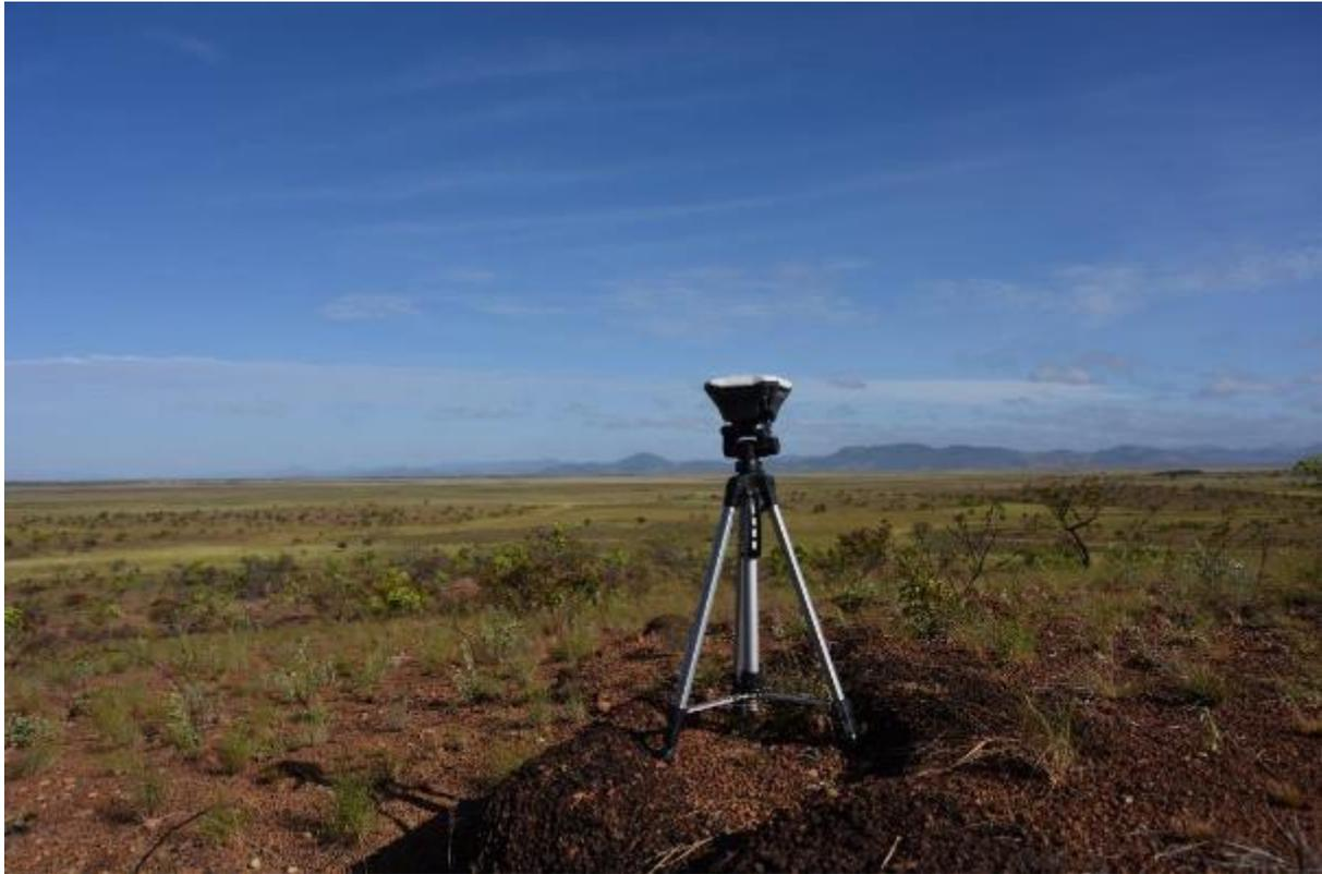
Figure 8: The RTK base station positioned at a point of high elevation overlooking the Rupununi Portal region in February 2018, at the height of the dry season. The same view during the wet season would show a transformed wetland landscape.
