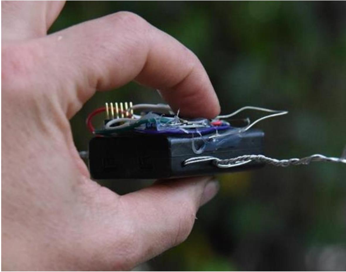
Figure 23: LoRa tracker unit before being encased in maritime epoxy.
