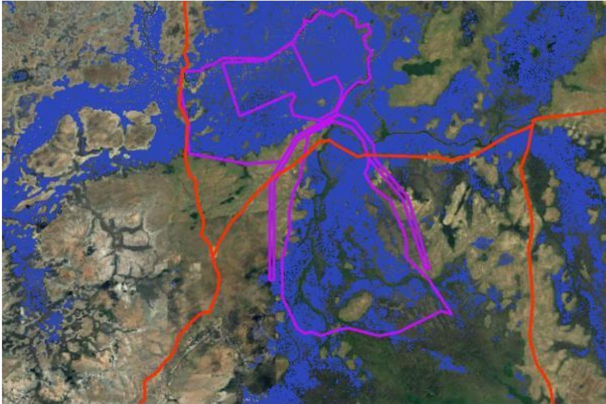
Figure 26: Footprint of the proposed Agricultural Centre and associated reservoir on the 2017 flood extent.
