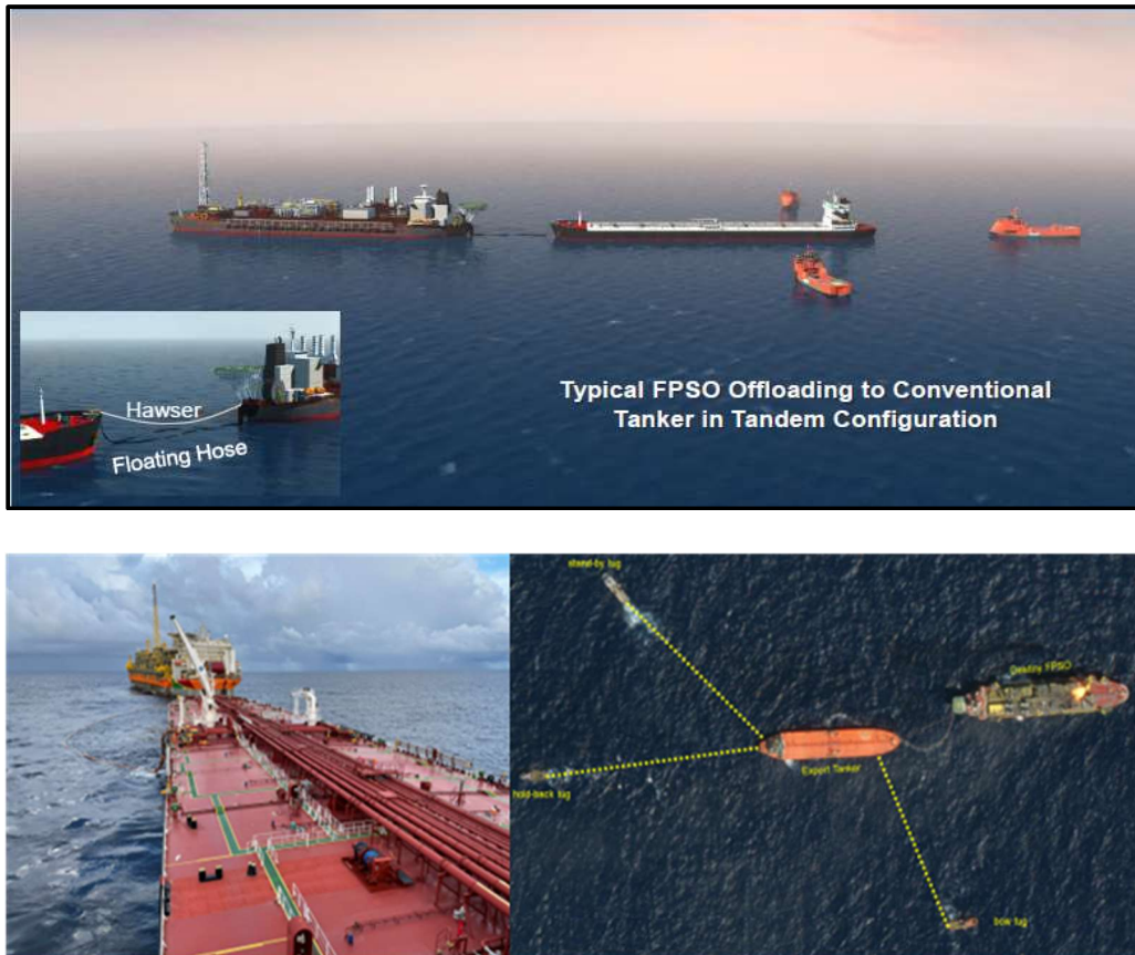
Figure 11: Tandem Offloading Configuration
