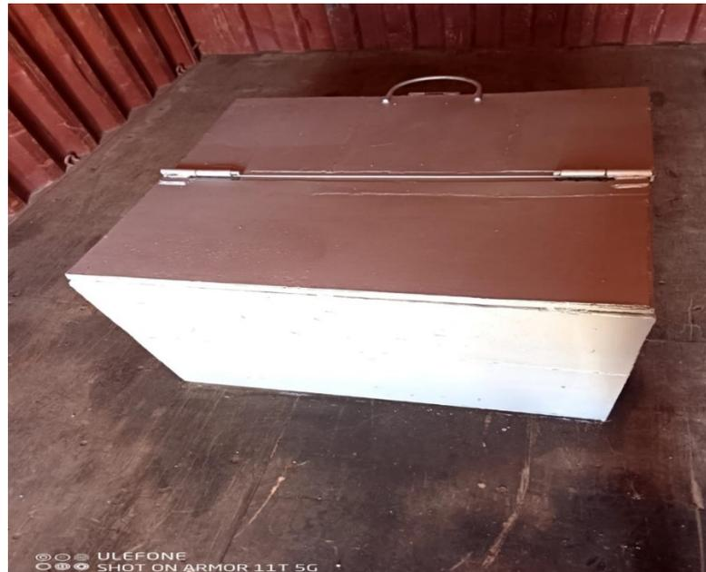
Figure 2: The Lead Lined Storage Box
