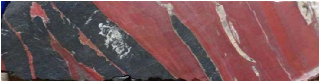
Figure 9-6: Alternating Bands of Braunite (Black) and Spessartite-Rich Purple Phyllite Forming Typical BMF Protore
