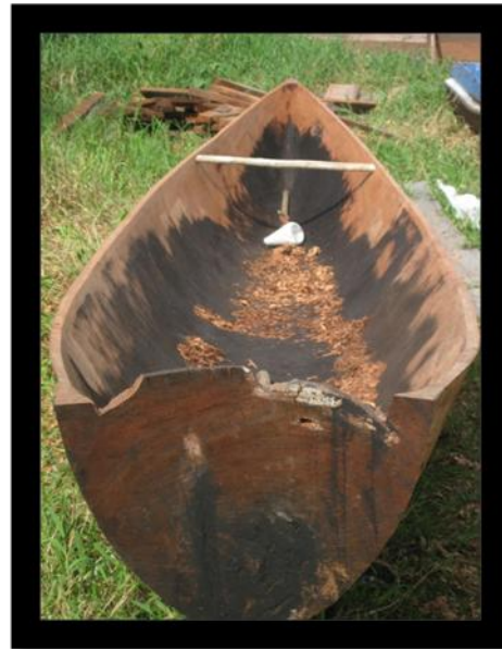
Fig 2: A traditional corial made from a single tree
