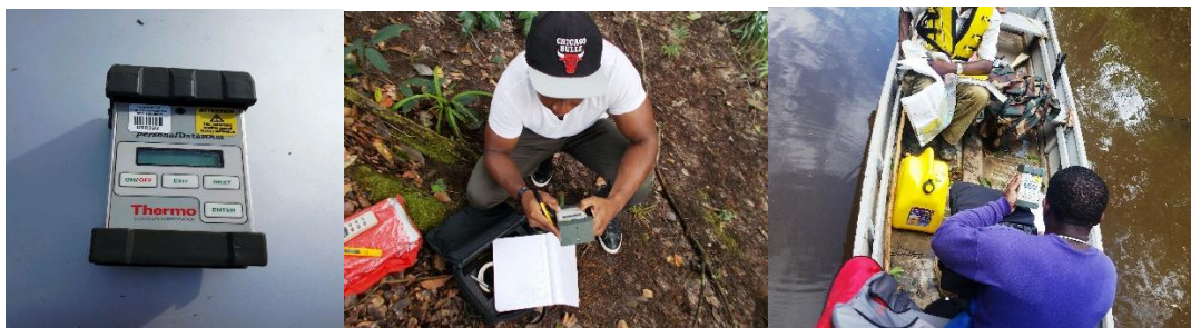
Figure 21: Air quality monitoring using a Thermo pDR-1000AN personalDataRAMTM Particulate Monitor
