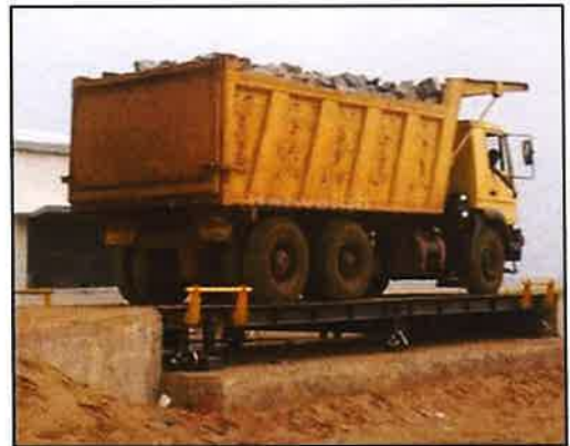
Photo 13: Fully loaded 30 tons’ truck being weighted on a scale.
