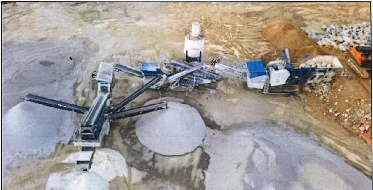
Photo 11: Crushers and screeners line, and classified aggregate rock stockpiles.
