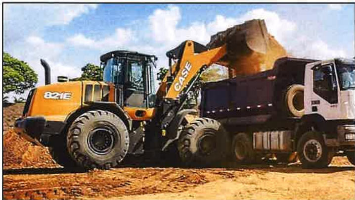
Photo12: Front-end loader loading 30 tons’ truck for off-site transportation.
